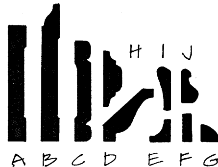
Types of molding shapes. A) base; B) base with integral ogee cap; C) chair rail; D) crown; E) cove; F) lattice; G) quarter round; H) astragal; I) picture; J) base cap.
