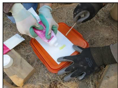
Akepox 2010 epoxy being squeezed out at a 2:1 ratio.
